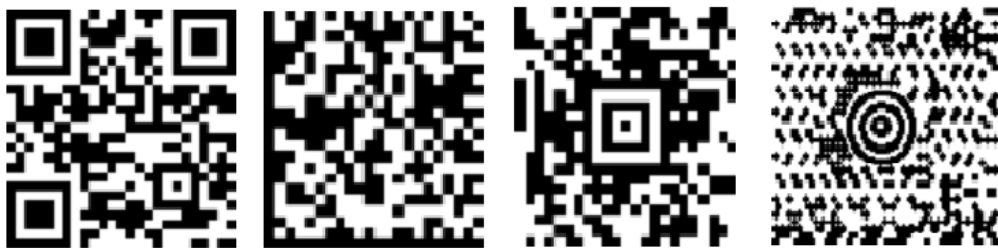
a) QR (Quick Response) code b) Data Matrix code c) Aztec Code d) MaxiCode
