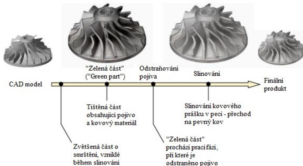
Obr. 20. Princip technologie atomic diffusion additive manufacturing. [30]
