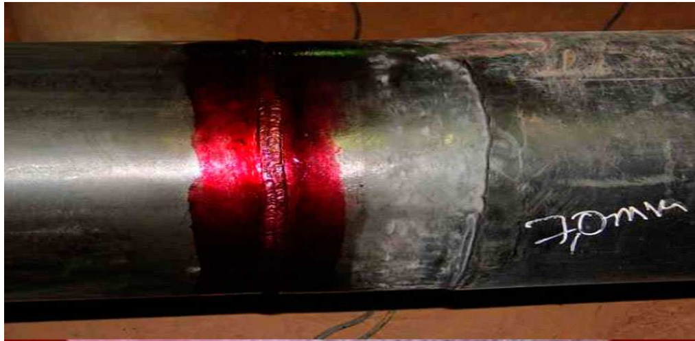
Fig. 45 Liquid penetrant inspection of pipe
