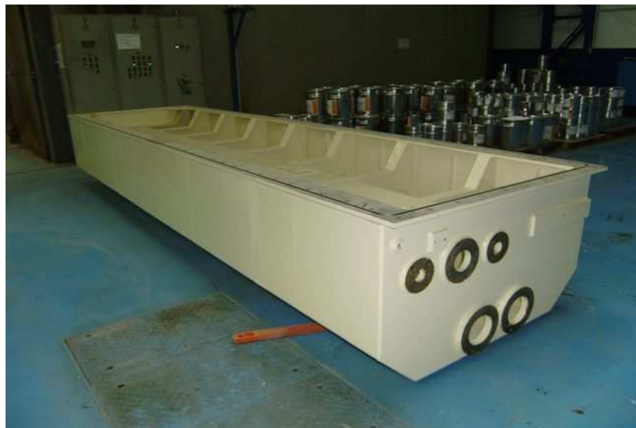
Fig. 49 Welded oil sump 102225
