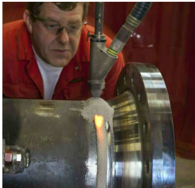
Fig. 20 Demonstration from welding submerged arc welding
