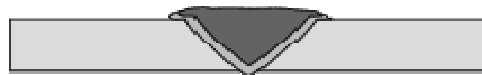
Cross section of a completed weld. The edges of the metal plates and molten filler rod have fused together to form the join.
