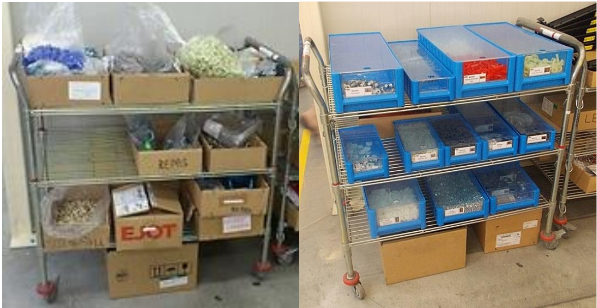
Figure 51: Standardized rack of Advanced preparation workplaces before (left) and after (right)
