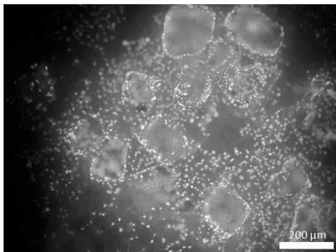
*Fig. 12 Cell growth on native CBS with 30% of space holder with grain sizes greater than 250  $\mu\text{m}$*
