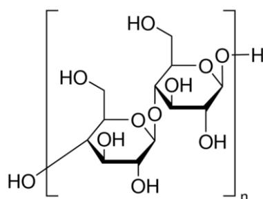
Fig. 5 Chemical structure of cellulose (“Cellulose C6288, Sigma-Aldrich,”)
