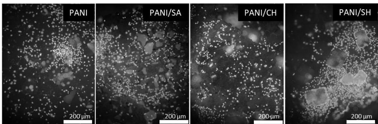
*Fig. 14 Cell grow on a modified ceramic scaffolds (CBS with 30% of space holder with grain sizes greater than 250  $\mu\text{m}$ ) under static cultivation (supplementary material of **ARTICLE I** (Martinková et al., 2022))*
