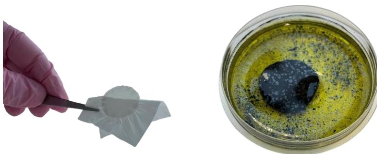
*Fig. 11 CNF-DAC disk on vapor permeable membrane after drying (left), CNF-DAC PPy after polymerization before washing (right)*
