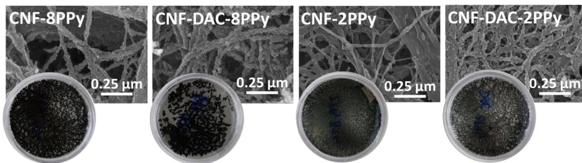
*Fig. 18 SEM analysis of CNF-2PPy, CNF-DAC-2PPy, CNF-8PPy, CNF-DAC-8PPy after 30 min of sonication, demonstrating PPy layer damage in samples of the CNF-PPy series; Petri dishes with samples after sonication to compare fragmentation of samples after sonication*
