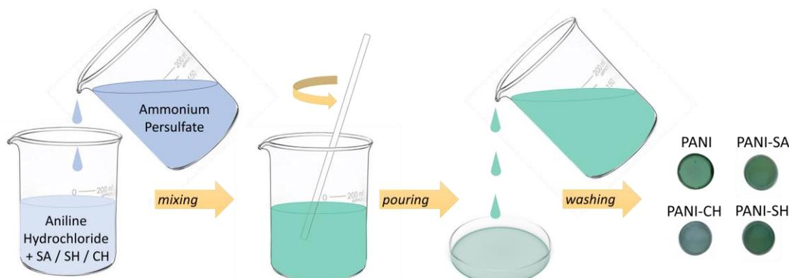
*Fig. 10 Scheme for the preparation of PANI films in colloidal dispersion mode stabilized by SA, SH or CH*
