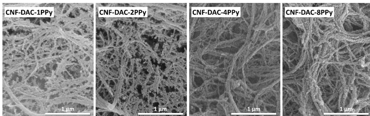
Fig. 17 SEM photographs of CNF-DAC with four different concentration of PPy
