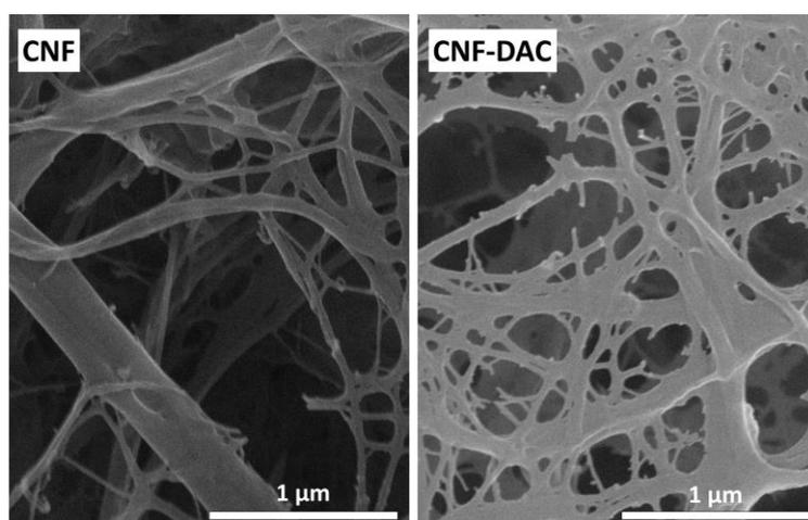
Fig. 16 SEM photographs of CNF and CNF-DAC suspensions
