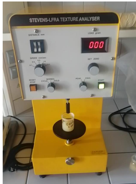
Figure 11. Machine for measuring the Bloom value in our laboratory.
