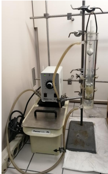
Figure 18. The viscosimeter for measuring the dynamic viscosity of the gelatines.
