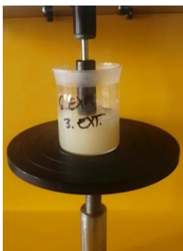
Figure 16. Measuring of Bloom value. Figure 17. The prepared gelatine gels for gel strength measurement.
