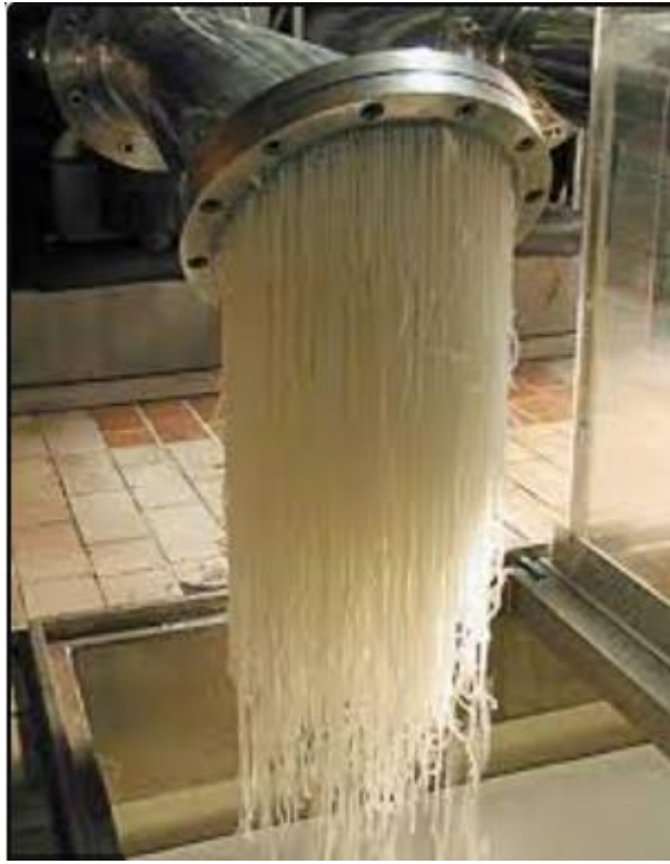
Figure 8. Extrusion of gelatine noodles. [41]
