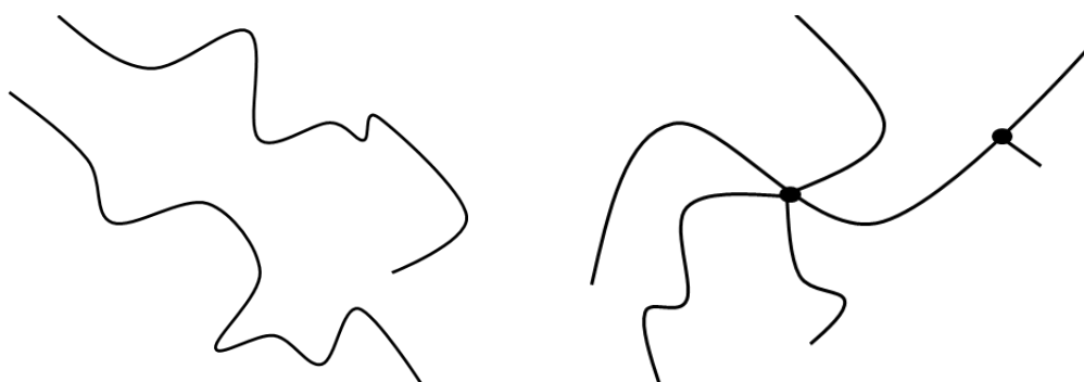
Fig. 15: Linear (left) and branched structure (right) of PP
