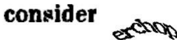
Fig. 17: CAPTCHA. The image was presented as a HIP when creating a new email account. It contains two strings, “consider” and “erchop.” Characters in the second one are warped (elongated and purposefully not following a straight line) to break attempts at automated analysis which would allow to create a valid account.
