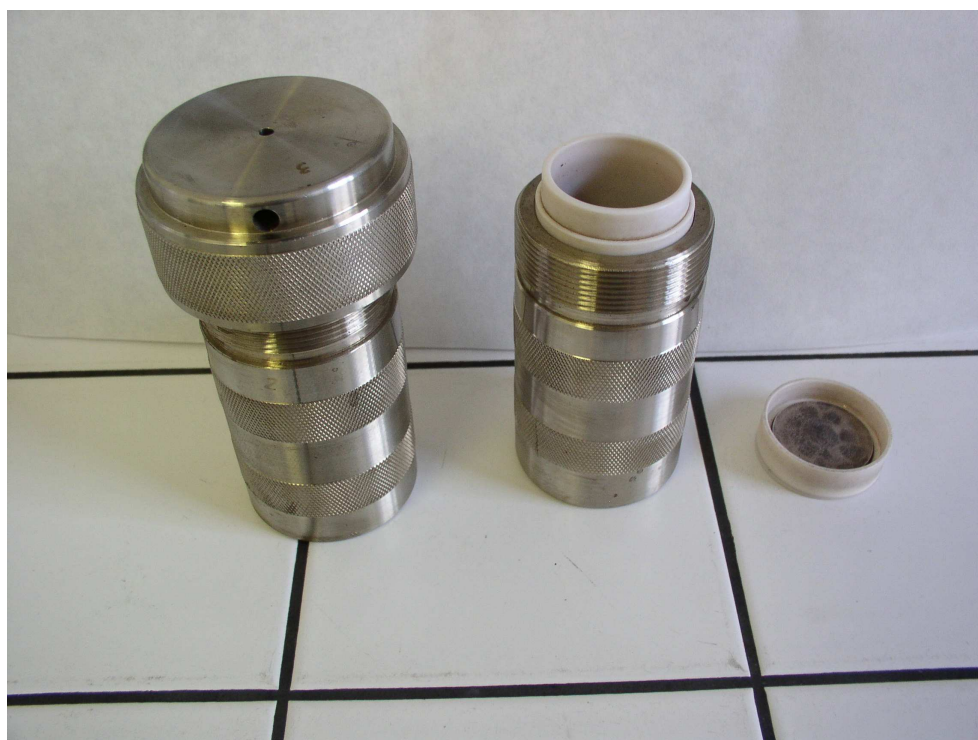
Fig. 22: Steel autoclave for preparation of TNt nanorods
