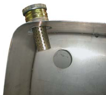
Obr. 30. System na ochranu nafty [12]
