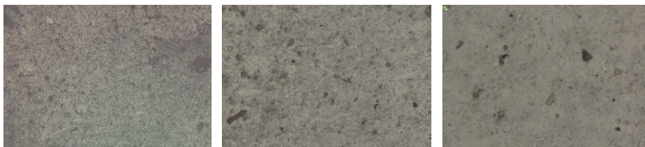
Figure 25: 80x (left), 200x (middle) and 400x (right) magnified crosslinked sample degraded under WG filter for 100 h – GA_200h
