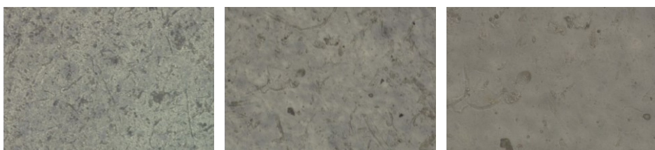
Figure 23: 80x (left), 200x (middle) and 400x (right) magnified crosslinked non-degraded sample – GA_0h
