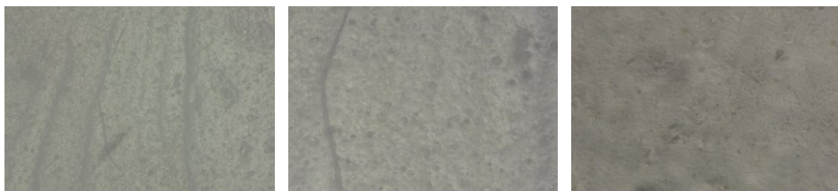
Figure 22: 80x (left), 200x (middle) and 400x (right) magnified non-crosslinked sample – 0h_Gly
