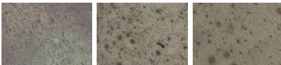
Figure 24: 80x (left), 200x (middle) and 400x (right) magnified crosslinked sample degraded under WG filter for 200 h – GA_100h
