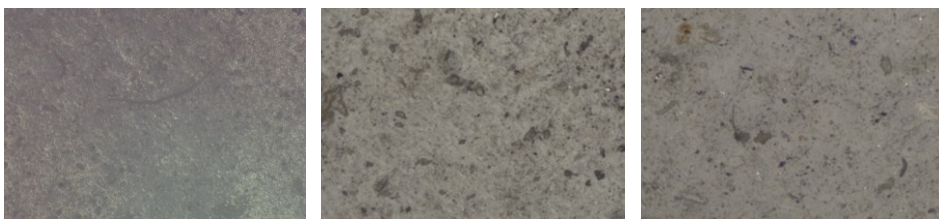
Figure 28: 80x (left), 200x (middle) and 400x (right) magnified crosslinked sample degraded under SL filter for 300 h – SL_300h
