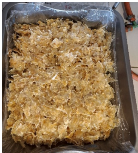
Figure 4: Defatted raw material ready for gelatin extraction.
