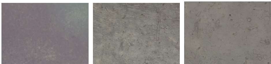
Figure 27: 80x (left), 200x (middle) and 400x (right) magnified crosslinked sample degraded under SL filter for 100 h – SL_100h
