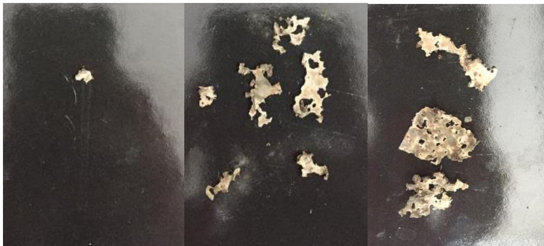
Fig 11. From left to right: PHB treated with air, PHB without treatment, and PHB treated with argon
