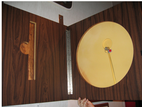
Fig. 1.4 The seal opened to reveal the hidden microphone [29].
