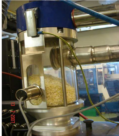
Figure 34. Mixed material in hopper
