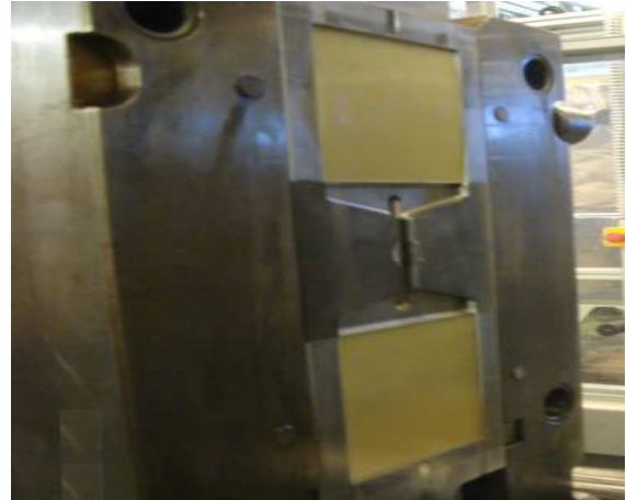
Figure 22. Prepared mould for overmolding
