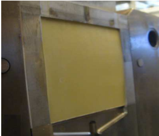
Figure 21. Inserted first layer into mould
