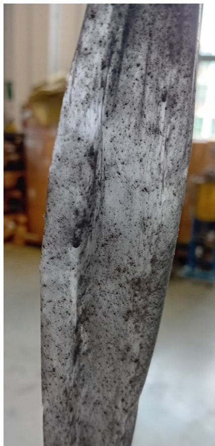
Figure 7: Photo of poor GO 2 filler dispersion in TPU matrix (left picture)
