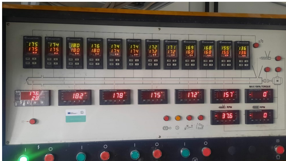
Figure 4: Extrusion conditions of TPU 11T80 with MMT fillers
