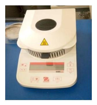
Figure 11 Moisture analyzer
