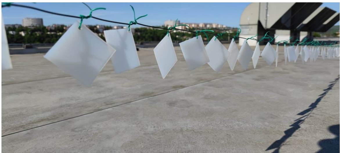
Figure 13 Detailed photo of the samples on the roof, exposed to natural aging
