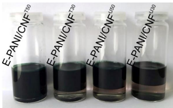
Figure 14 Creaming of Pickering emulsions with undecane (U) and caprylic/capric triglyceride (T) oils stabilized with PANI/CNF: E-PANI/CNF T50 ; E-PANI/CNF T30 ; E-PANI/CNF U50 ; E-PANI/CNF U30 after preparation.
