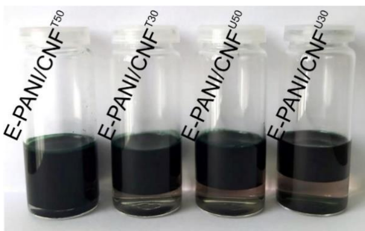
Figure 44 Creaming of Pickering emulsions with undecane (U) and caprylic/capric triglyceride (T) oils stabilized with PANI/CNF: E-PANI/CNF T50 ; E-PANI/CNF T30 ; E-PANI/CNF U50 ; E-PANI/CNF U30 after preparation.
