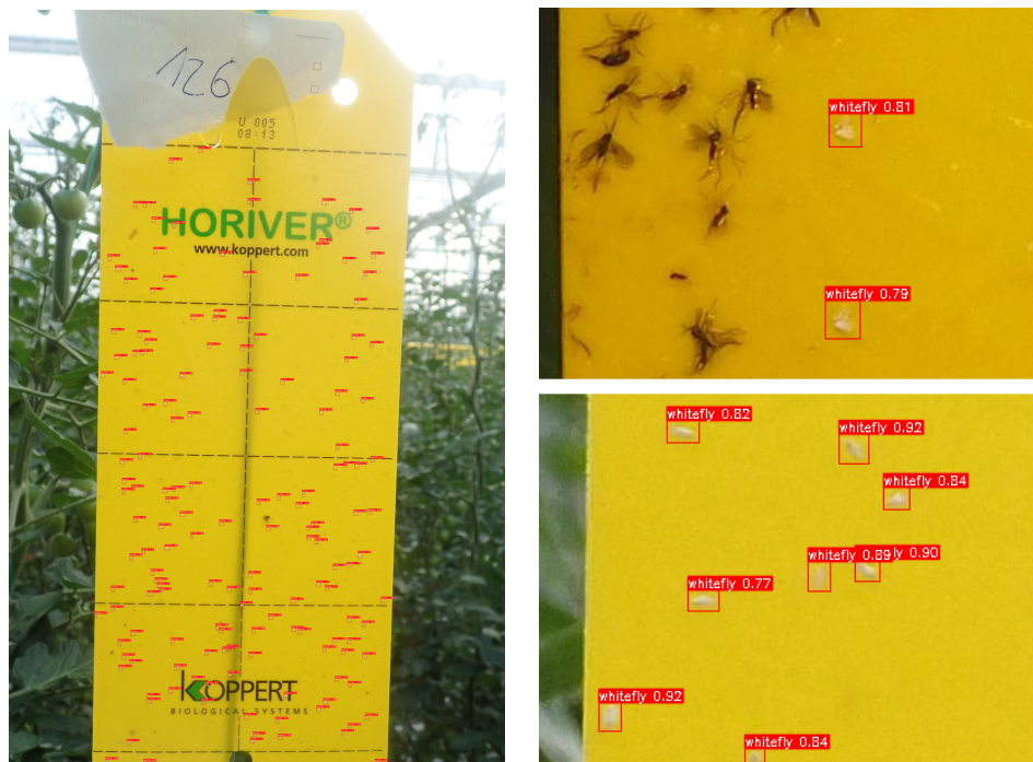
Fig. 5.7 On the left side is the example of the full input image with bounding box detections (red boxes) marking present whiteflies. On the right side, there are the zoomed cutouts with bounding box detections marking class labels and the model's detection confidence.
