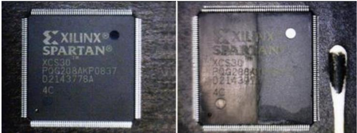
Figure 6 Heated Solvent test reveals blacktopping
