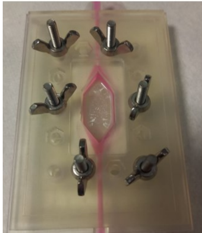
Figure 36 The removable part of the chamber with residues of nanoparticles after dynamic cultivation.
