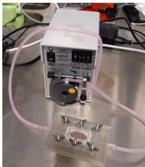
Figure 35 Closed system. To avoid sedimentation, the reservoir bottle was removed from the scheme, so the full volume of liquid was moving.
