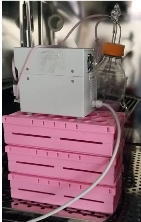
Figure 33 Reservoir bottle on an orbital shaker in the incubator. To prevent the sedimentation of nanoparticles, a reservoir bottle with suspension was put on to orbital shaker in the incubator.
