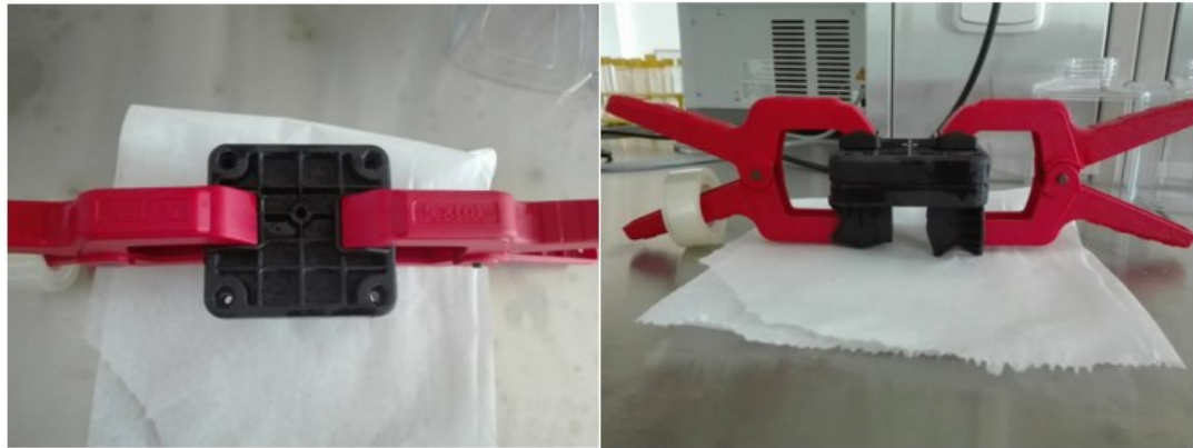
Figure 43 Mold with PDSM secured with clips to protect the PDMS from leaking out.
