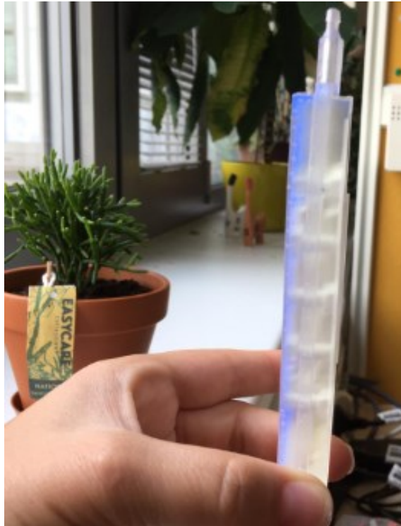
Figure 27 The dynamic flow chamber on sunlight. The material from which was chamber made reflected the sunlight and was not suitable to observe directly under the microscope.
