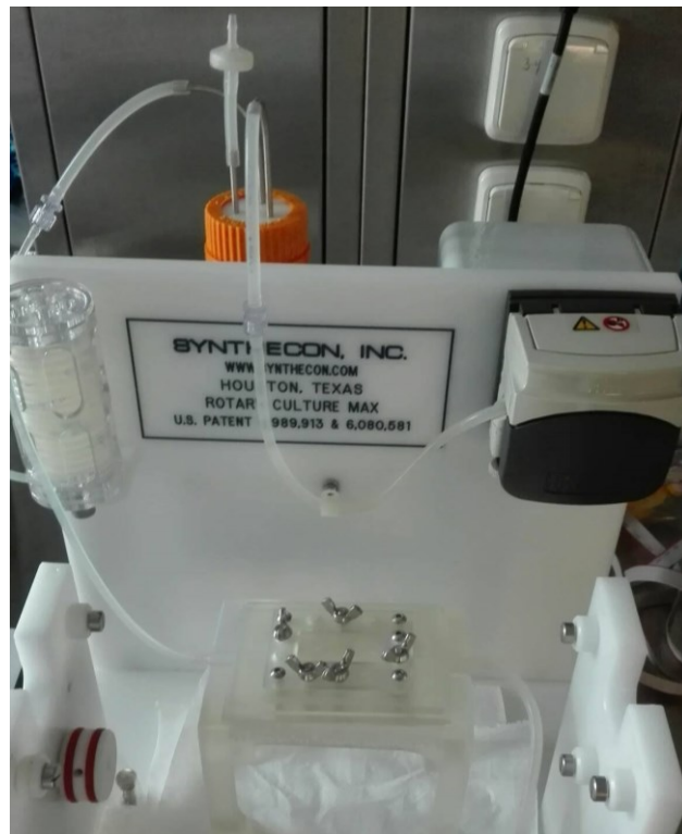
Figure 25 The dynamic flow chamber. The chamber is assembled together with pump, reservoir bottle and oxygenator.
