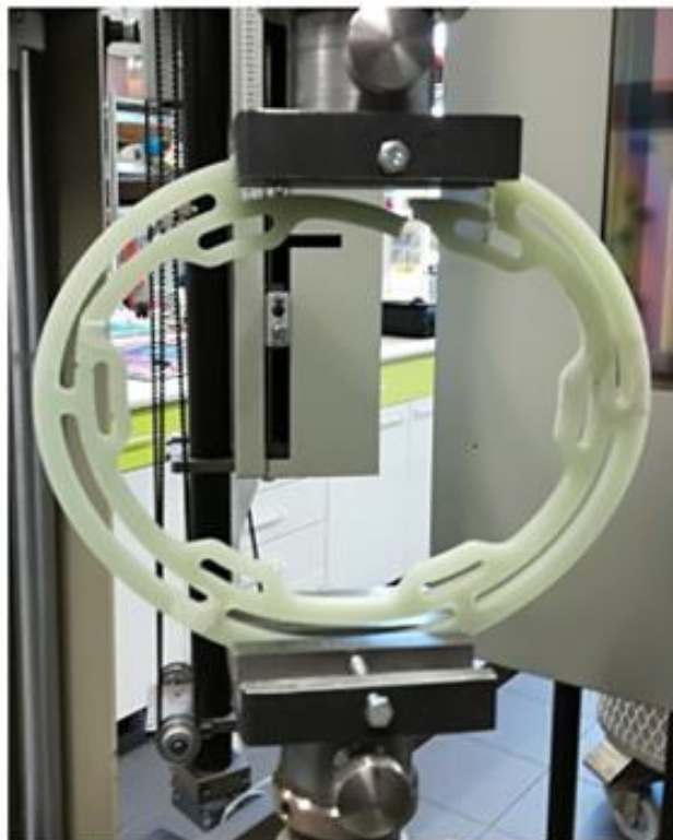
Fig. 11.11: Fixator ring with fracture after the loading process
