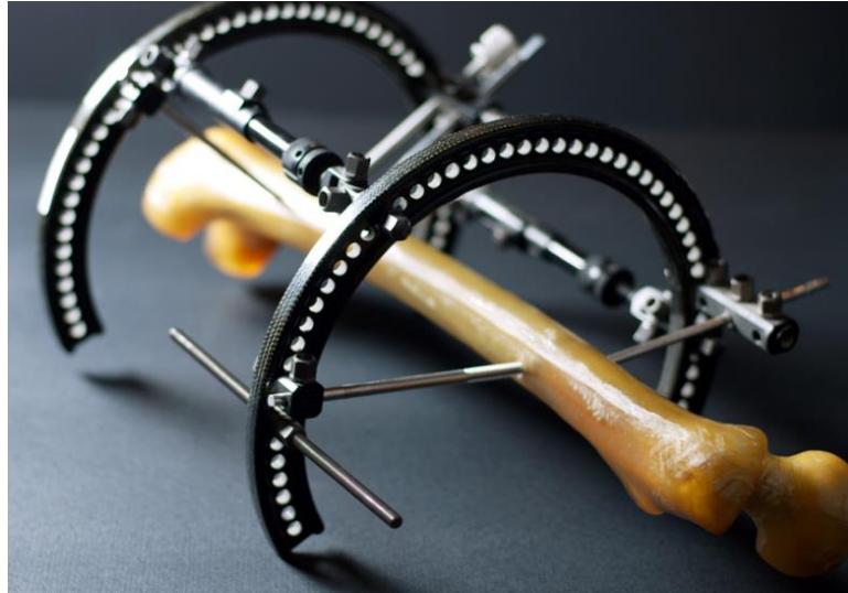
Fig. 4.4: Assembly of a composite external fixator with polymer bone [84].
