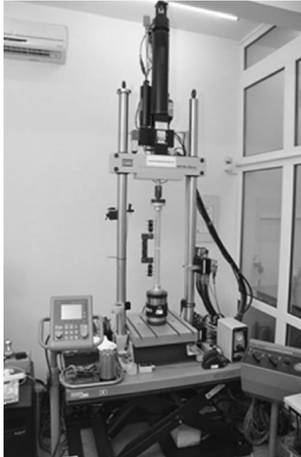
Fig. 6.2: The testing system for external fixator loading
