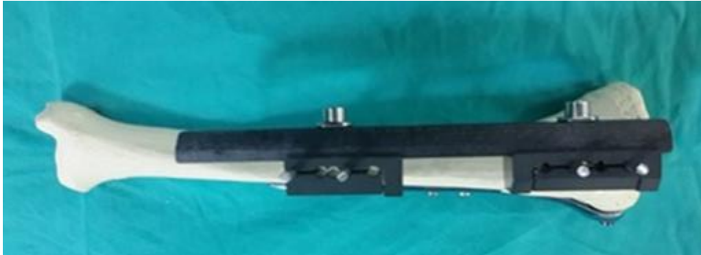
Fig. 4.5: Composite external fixator with polymer tibial bone [85].
