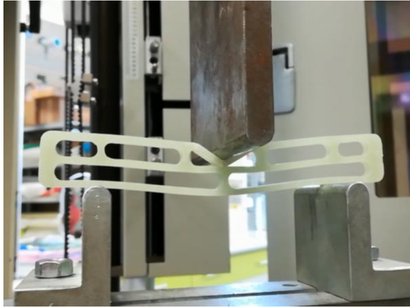
Fig. 11.10: Composite sample – version 6 during the process of three - point bending
