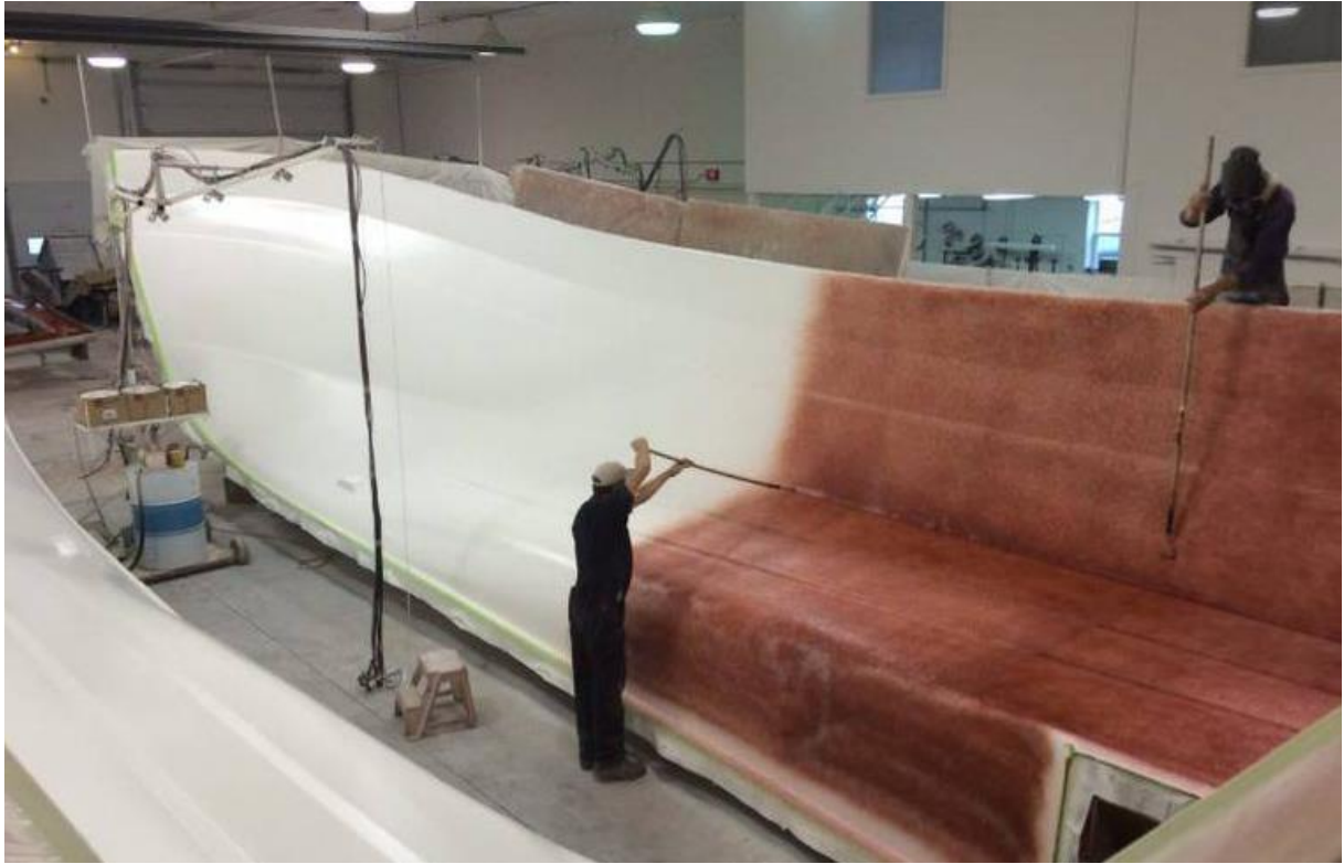
Fig. 4.7: Manual lamination of boat [124]
