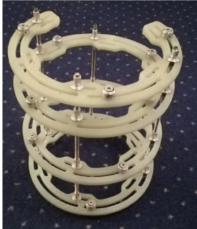
Fig. 12.7: Assembled external fixator with composite rings
