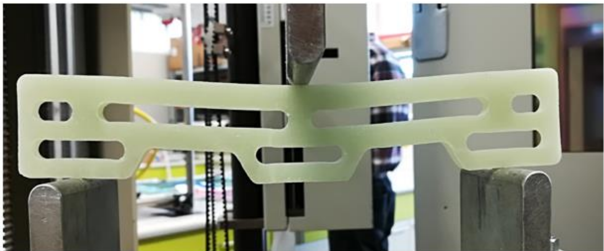
Fig. 11.6: Loading of the specimen by the three-point bending in the first direction
