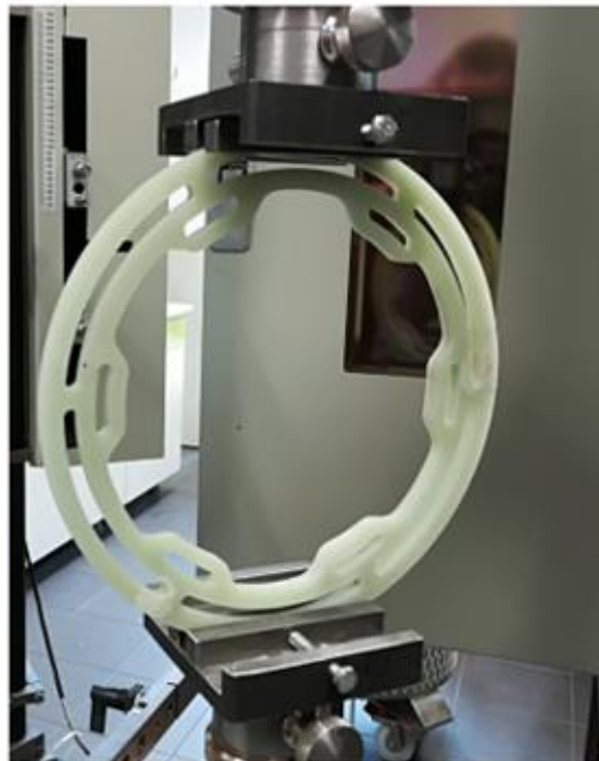
Fig. 11.8: Loading of the specimen by the pressure
