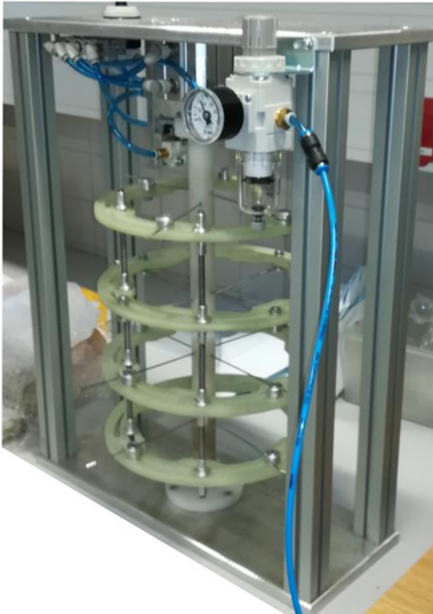
Fig. 13.6: Cyclic testing machine manufactured by Matěj Homola connected with the manufactured external fixator
