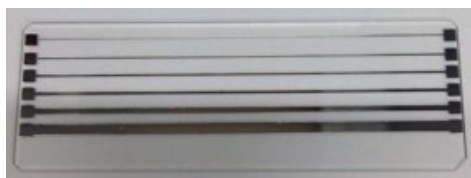
Fig. 5: Ink-jet printed silver lines array of pixelated geometry as 1, 3, 5, 10, 20 and 40 pixels. Length of 71 mm was kept constant
