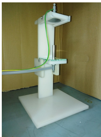
Fig. 10: Electrospinning device used in experimental part of the current thesis (high voltage power supply not in picture)
