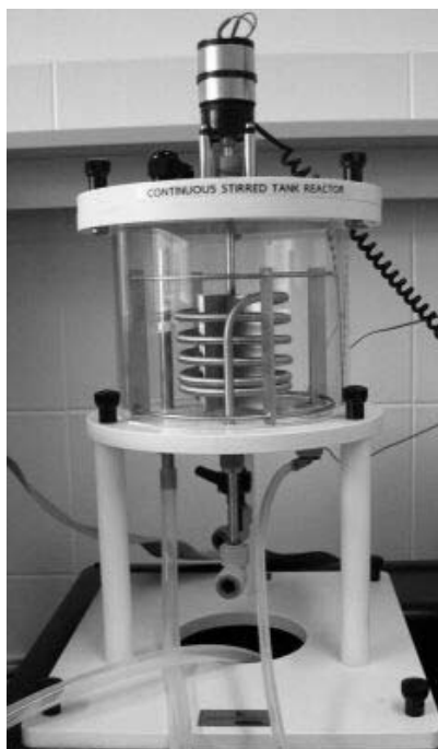
Figure 4.46 PCT41 and PCT 42 – Process Vessel Accessory (CSTR)
