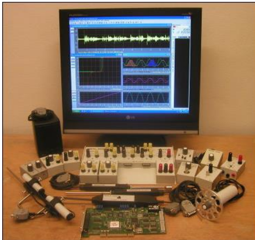
Figure 1 ISES physical hardware and software components; the PCI ADDA converter, the set of meters, sensors and device
