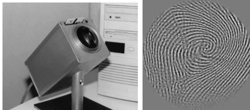
2.6 Ultrasonic reader – Optel Ltd R&D model of ultrasound camera; Picture taken by an ultrasound reader [7]
