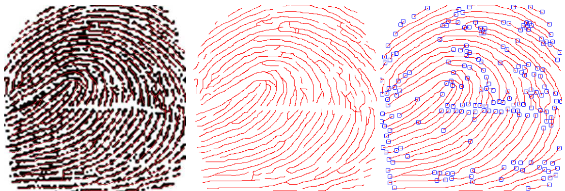
3.4 Ethalon1 with a wire model; wire model; wire model with a markant map
