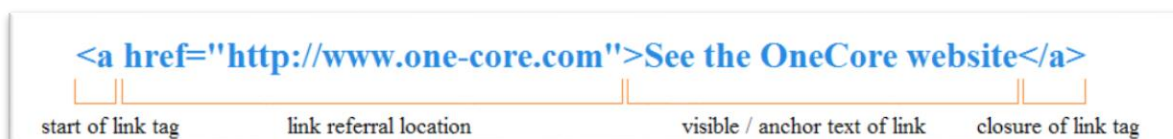
Figure 3 – Anatomy of a link (own processing)
