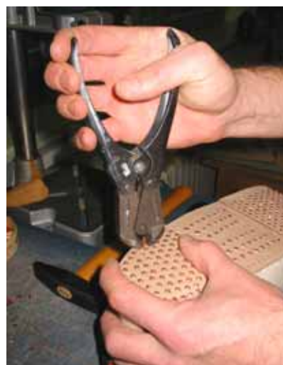
Fig. 52. Shortening the length of a peg
