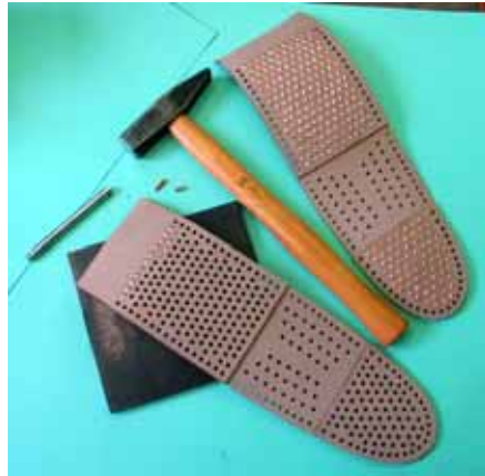
Fig. 48. Fitting the pegs into the holes on the sole
