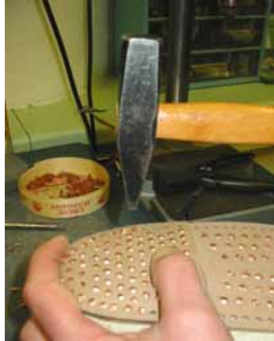
Fig. 54. Forming a head of a peg with a hammer
