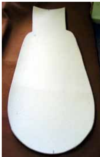
Fig. 42. Pattern of the main upper part
