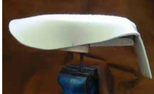
Fig. 45. Upper material attached to the last
