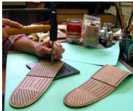
Fig. 49. Forming the pegs on the sole
