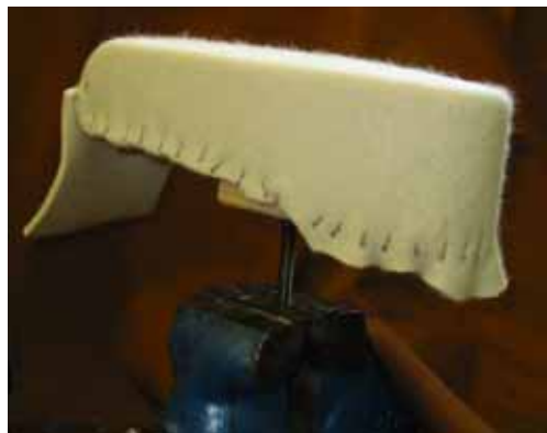
Fig. 46. Formed upper fixed on the last by nails
