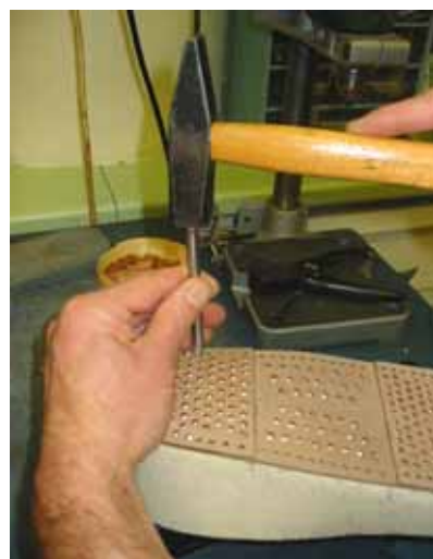
Fig. 53. Forming a head of a peg
