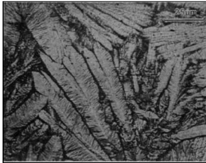
Fig.I. 11 Reflection optical micrograph of lamellae in isotactic polypropylene arranged in feather-like structures. The polypropylene sample was crystallized isothermally at 203°C and 200 MPa and was permanganically etched for 30 minutes.
