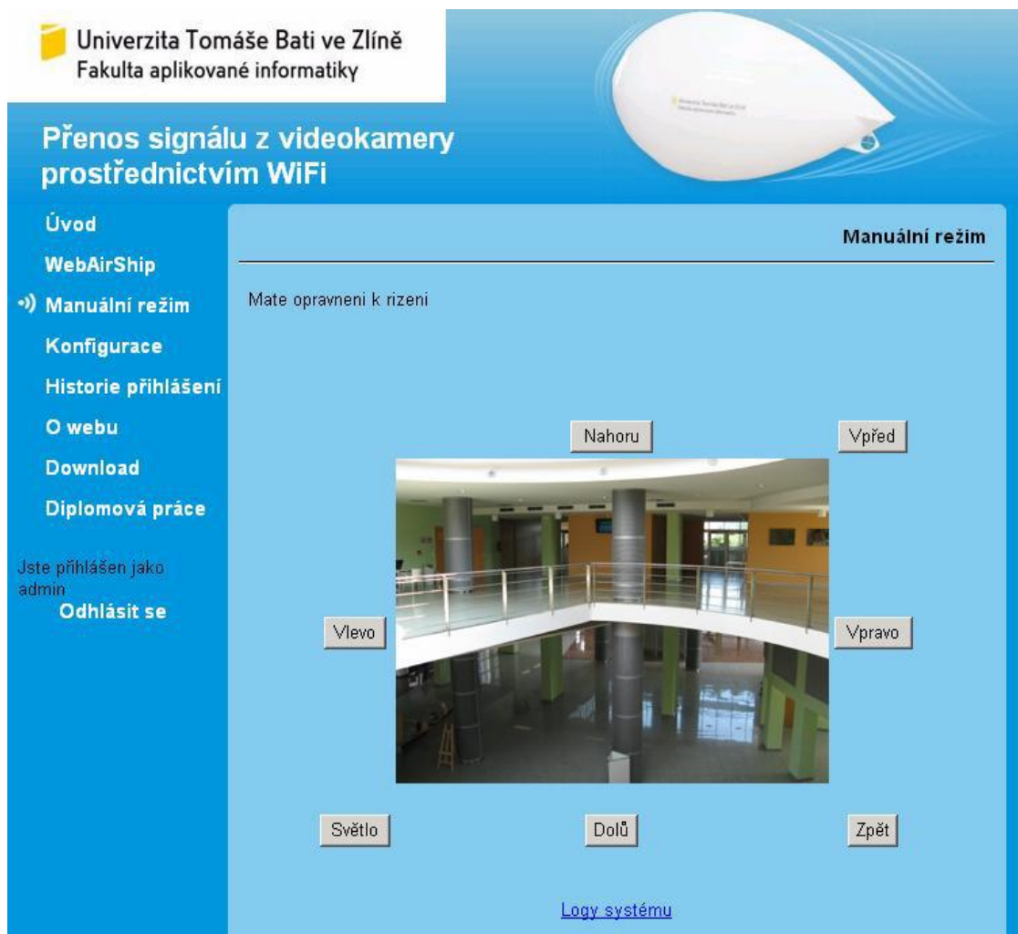
Fig. 60 – Autonomous monitoring system web interface – manual control mode
