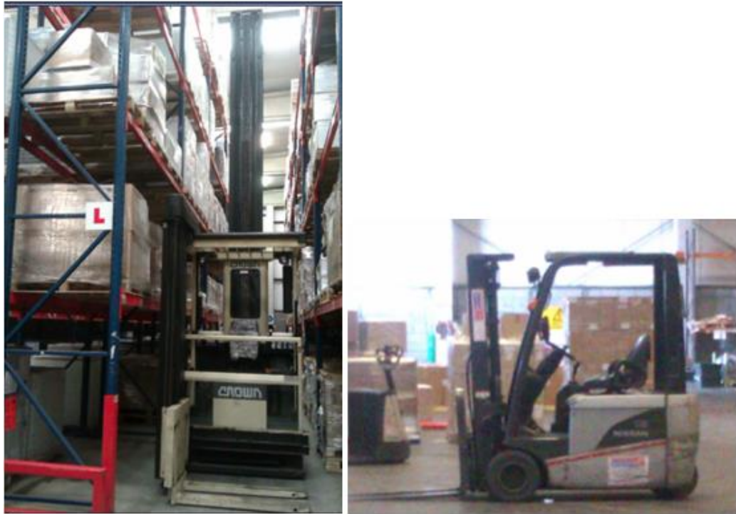
Figure 50: Turret Truck and Forklift used at W/H
