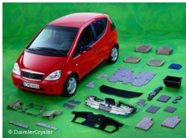
Figure 5 Indoor applications of natural fibre reinforced polymers in Mercedes Benz Class A [25]
