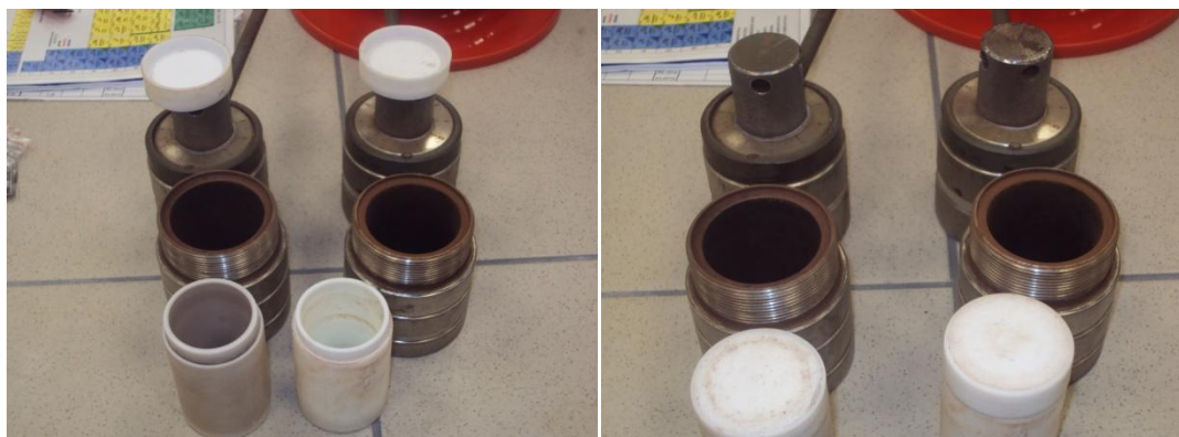
Fig. 1. Images of autoclaves used for solvothermal synthesis.
