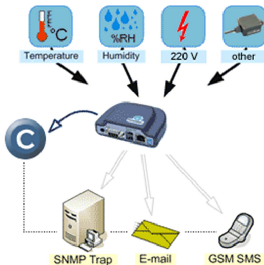
Obr.25 IT monitoring system
