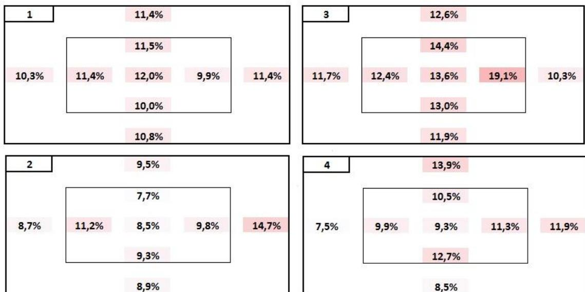
Figure 28. Moisture profile of “dry” bale (1.05), ref. No. 101124.
