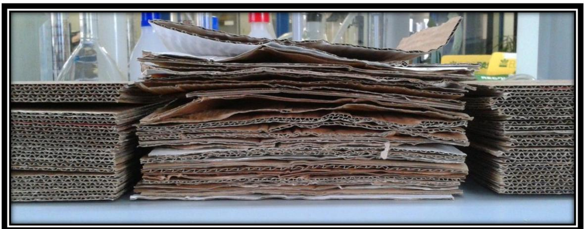
Figure 46. Sheet board samples – recovered board in the middle and virgin board on sides.
