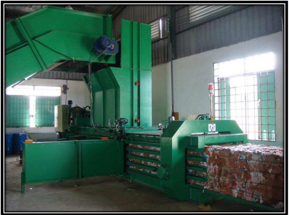
Figure 24. Horizontal waste paper baling press – Techgene Machinery Co., Ltd.
