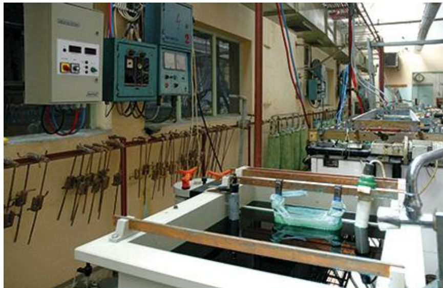
Figure 68 Department for manufacturing galvanic molds from nickel
