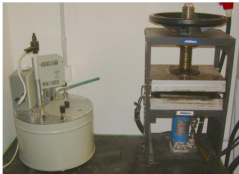
Figure 76 Thermostat for cooling and hydraulic press
