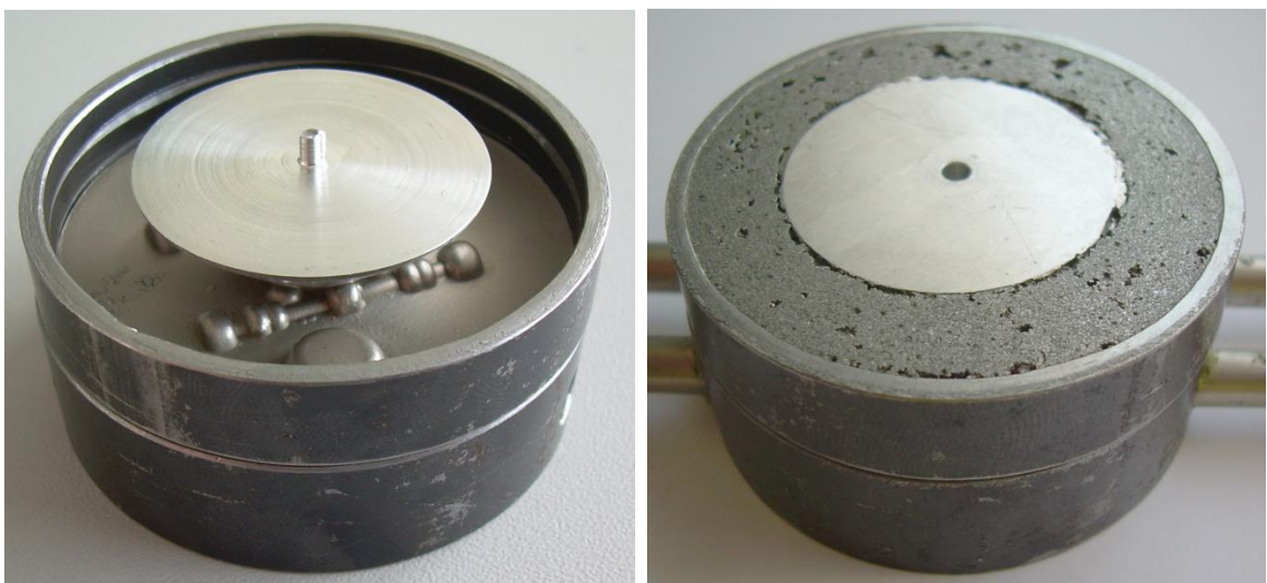
Figure 72 Sprue and supporting ring filled by epoxy resin with aluminum powder
