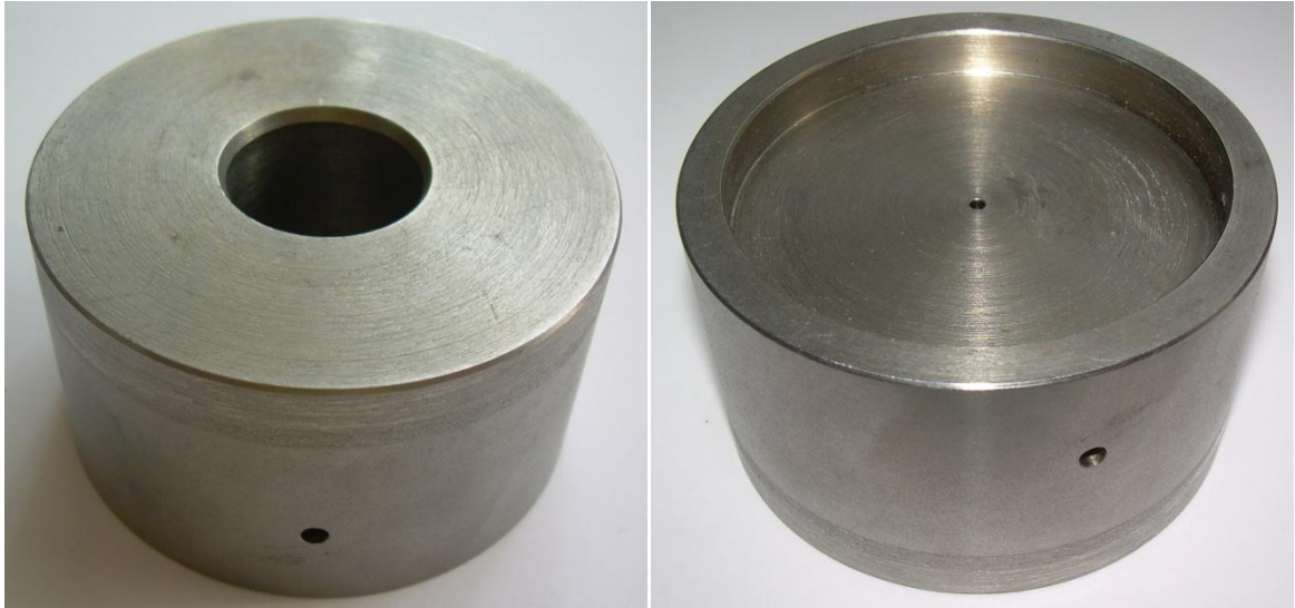
Figure 73 Front and back side of the transfer pot
