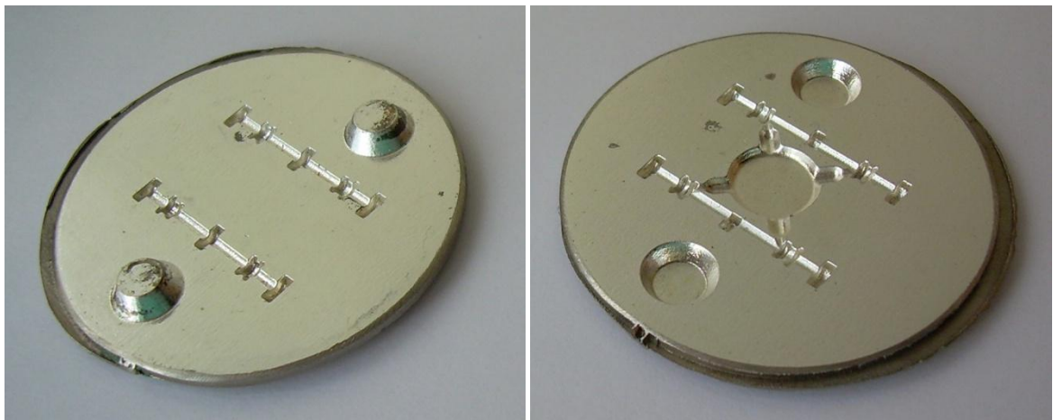
Figure 69 Nickel cavity plates produced by electroforming
